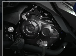
Engine SOHC, 4 Valve, 185cc. Biggest displacement in its category.
