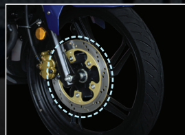
Brake Disk Large brake disk in its class with 250mm diameter
